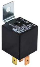
RE1008 Relay 12VDC Coil Current : 133mA Contact Rating: 2x15A 14VDC Standard Mini 896 Series
